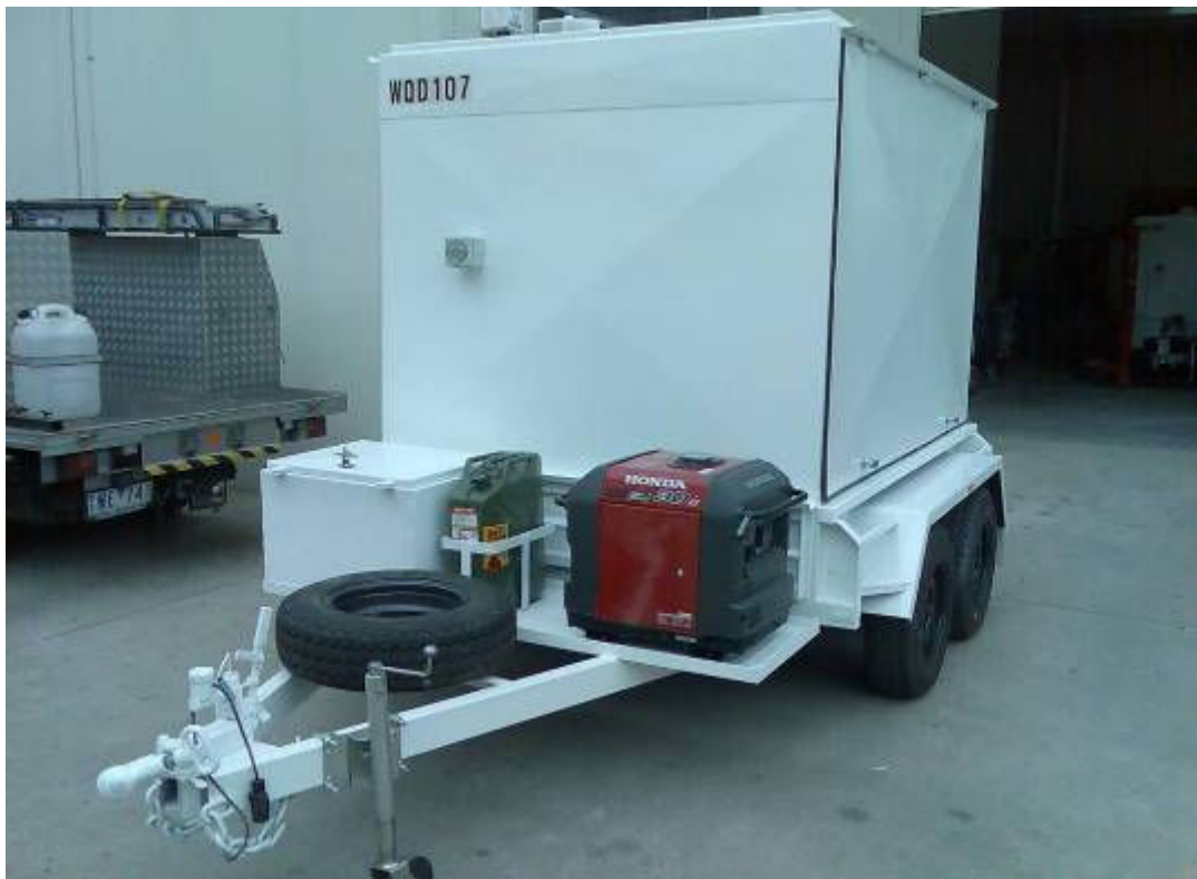
Photo 1 – Portable Dosing Unit (PDU)
